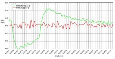
Fig. 6. Graphical representation of required and measured engine rotations
